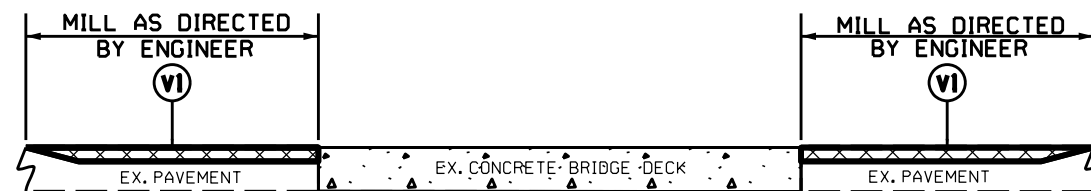
DETAIL 2 BRIDGE MILLING
